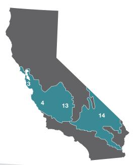
Effective January 1, 2023 gas instantaneous water heater (max input 200,000 Btu/h) installation is permitted in climate zones **3**, **4**, **13**, **and 14** if the space conditioning system is a heat pump.
