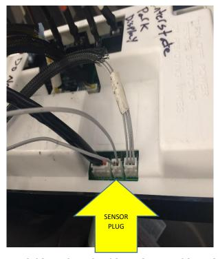
UNPLUG CONDESATE SENSOR FROM THE CONTROL BOARD
